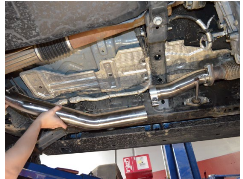
6. Connect the mid pipe to the front pipe. Secure using the provided 76mm clamps.
