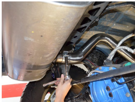
8. Connect the mid pipe to the OEM muffler and secure using the provided 66mm clamp.
