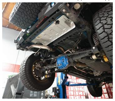
completed the installation of this exhaust system. Periodically, check the alignment of the exhaust, normal wear and tear can cause nuts and bolts to come loose. Note: Check clearance and adjust if needed! Failure to check the alignment and adjust the exhaust can cause damage that will void the warranty. Injen Technology is not responsible for any damages caused by/from improper installation.
