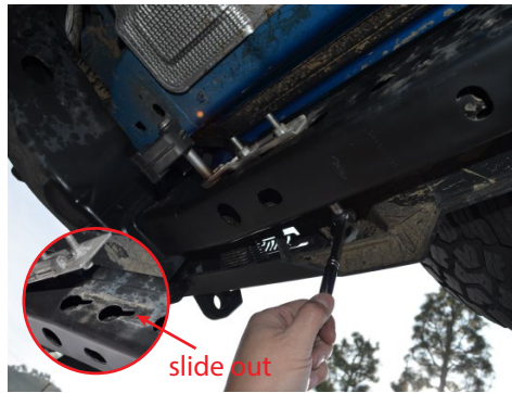
2. 2.3L MODELS ONLY: Remove the OEM hanger by loosening the two bolts and then sliding it out. The bolts can be accessed from the rear of the subframe.
