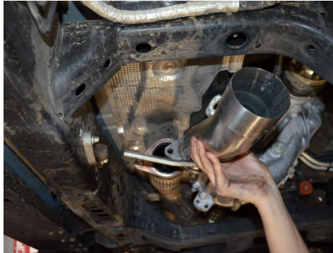
5. Connect the front pipe to the OEM flex pipe, then insert the hanger to the rubber insulator. Secure using the OEM nuts.
