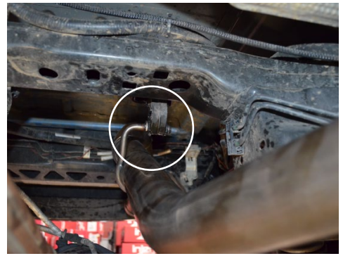
3. Detach the midpipe hanger from the rubber insulator.
