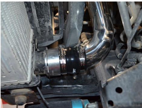
19. Once in position, secure all clamps on the 2.75" hump hose.
