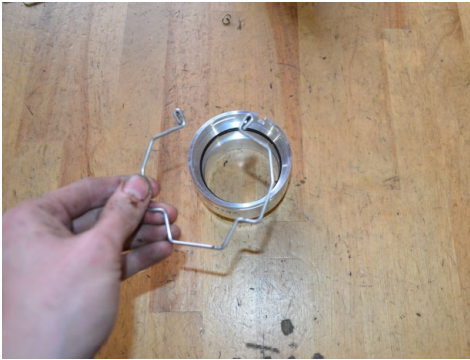
13. Install the retaining clip onto the intercooler adapter.
