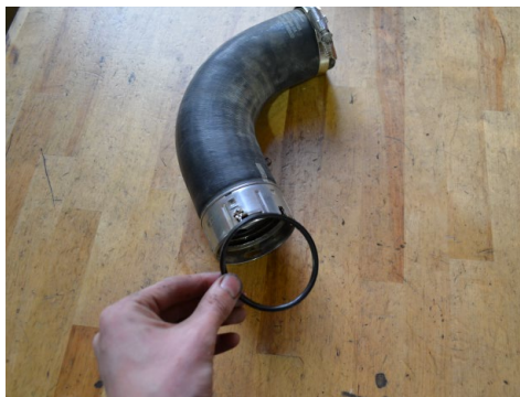
11. Remove the O-Ring from the intercooler hose. Note the direction it was removed in.
