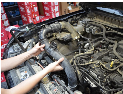
8. Remove the OEM intercooler pipe from the vehicle.
