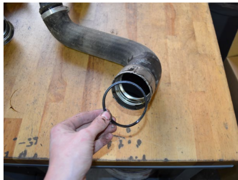
32. Remove the O-Ring from the intercooler hose. Note the direction it was removed in.
