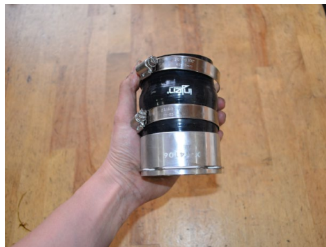
35. Install the 2.75" hump hose onto the intercooler adapter. Only secure the clamp on the adapter side.
