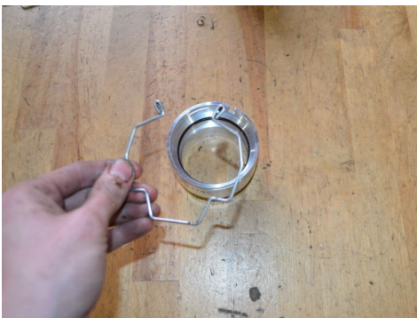
34. Install the retaining clip onto the intercooler adapter.
