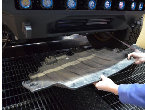
5. Remove the OEM skid plate.
