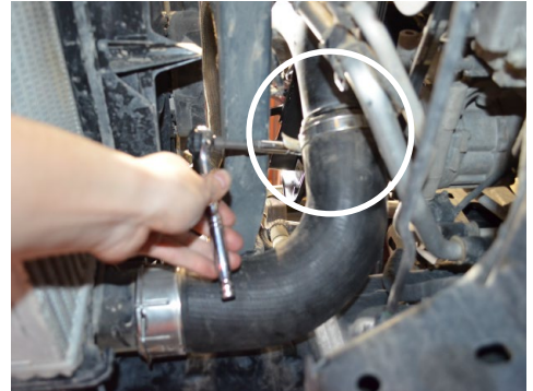
6. Loosen the clamp securing the bottom intercooler hose to the intercooler pipe.
