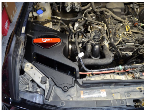
35. Reinstall the OEM intercooler pipe by following step 8-13 in reverse order. Once complete, ensure all nuts, bolts, and clamps are properly secured.
