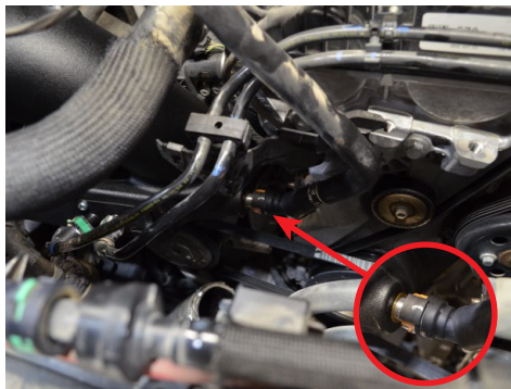
32. Reconnect the orange crank case line. A clicking sound will confirm it is properly secured.
