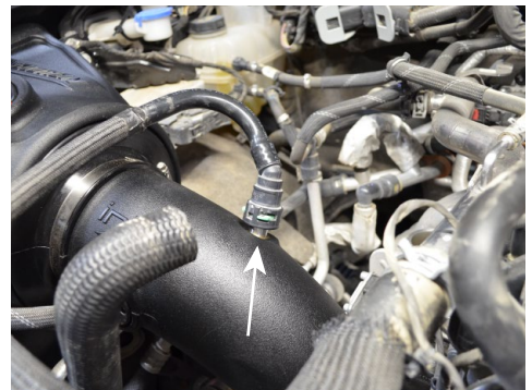
33. Reconnect the top crank case line. Once fully seated, ensure the green clip is locked into place.
