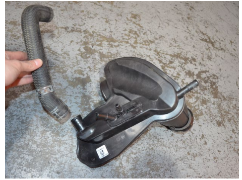
27. Release the tension clamp on the diverter valve hose then remove the hose from the OEM intake tube.
