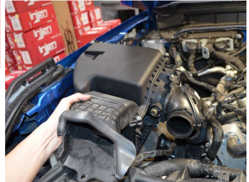
6. Firmly lift up on the air box assembly, then remove the air box assembly from the vehicle.
