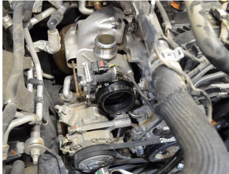
29. Attach the 2.50"-3.50" Stepping hump hose onto the turbo. Ensure the hose is properly seated before securing the clamp.
