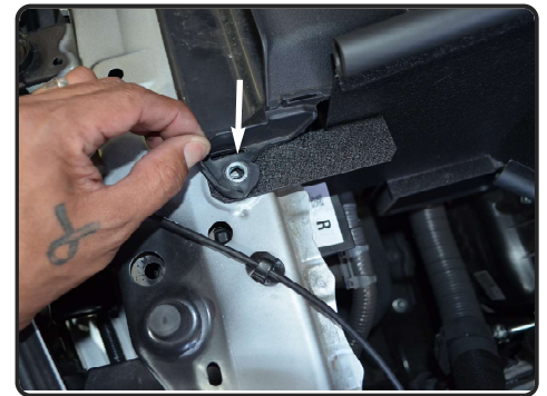
16. Place the tab under the ram scoop and tighten using OEM screw. Secure and tighten.
