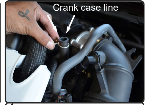
4. Push the factory clamp in and pull back the crank case line away from the intake tube.
