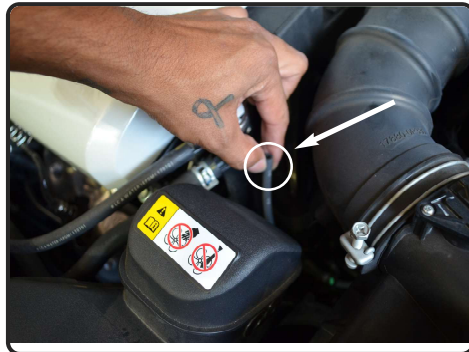
6. Pull back the vacuum line away from the intake tube.
