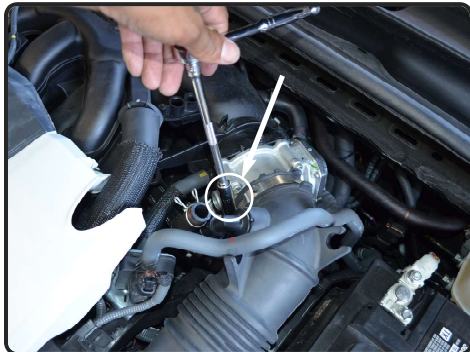
5. Loosen the clamp on the throttle body using 10mm socket or wrench. Pull back the intake tube from the throttle body.
