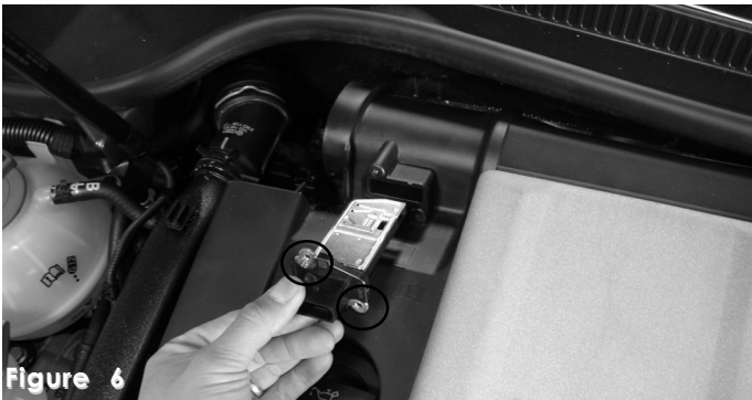
Figure 4 Remove the front plastic expanding plugs and torx bolt by the side battery base in order to detach the front air scoop.
