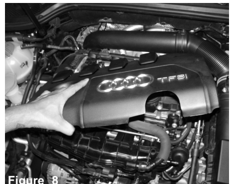
Figure 8 Remove engine cover.
