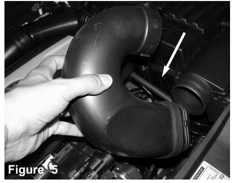
Figure 5 Pull out ram air elbow from air box.
