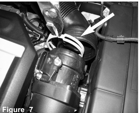
Figure 7 With pliers, carefully pinch clamp and pull intake tube away from air box.
