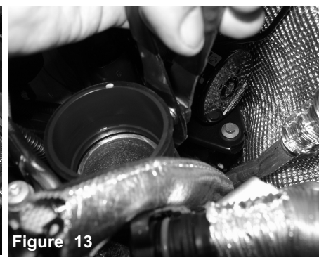
Figure 13 Pinch remaining clamp on turbo and remove.
