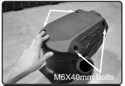
11. Place the following M6X80mm and M6X40mm bolts illustrated by the photo. Secure the bolts with a phillips head screw driver
