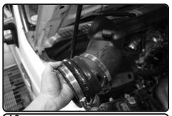
**16.** Place the 4.50" hump hose and two #72 clamps onto the big end of the Injen intake tube. You will have to slip the entire hump hose over the tube to make room to install the tube onto the Injen air box.
