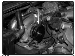
**15.** Place the 3.0"- 4.0" step hose with #64 and #48 clamps onto the turbo inlet. Secure only the clamp on the turbo side for now.
