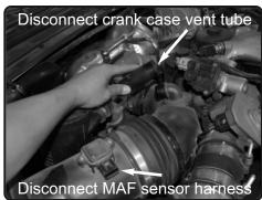
**3.** Disconnect the crank case vent tube from the factory air duct and MAF sensor harness from the MAF sensor on the air box assembly.
