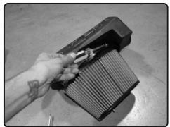
**9.** Place the filter onto the filter flange under the Injen air box plenum and then secure the clamp.
