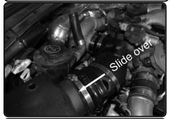
**17.** Push the 3.0" end of the Injen tube into the 3.0"-4.0" step hose on the turbo. Then slide the 4.5" hump hose over to the Injen air box side.
