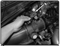
**5.** Unscrew the screws on the MAF sensor and then remove the MAF sensor from the factory air box assembly.
