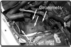
**12.** Locate the three factory air box mounting grommets. The Injen air box will also mount to these grommets. The air box inlet is also shown, which will insert into the Injen air box in the next step.
