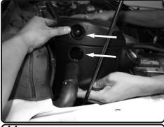
**14.** You can choose either port to con-nect the factory warm air tube. The open port is recommended for extremely cold weather.
