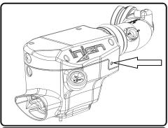
7. If equipped with an OEM filter monitor, drill a 1/2" hole located on the plenum indicated by the arrow. Reuse the OEM grommet to attach monitor to plenum
