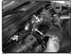
**4.** Loosen the two clamps on the factory air duct and then remove the entire factory air duct.
