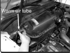
**6.** Detach the warm air tube from the factory air box assembly. Lift up firmly on the air box assembly and remove the air box assembly out of the engine bay.
