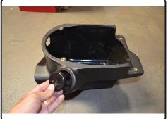
**8.** Place the Filter Minder plug into the lower air box assembly
