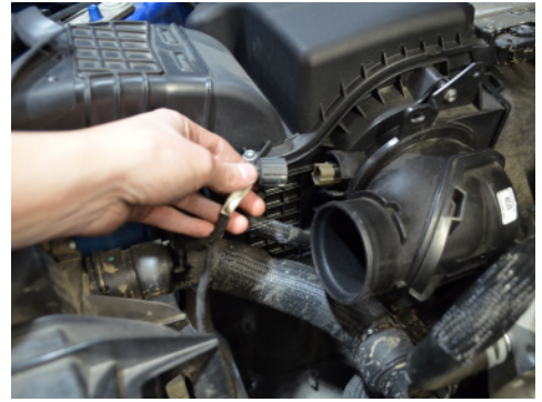
15. Disconnect the IAT sensor harness.
