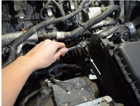
17. Loosen the clamp securing the passenger side tube to the air box.
