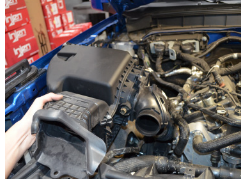
18. Lift the air box out of the engine bay.
