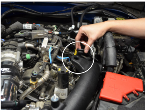
31. Install the OEM grommet onto the injen driver side tube.
