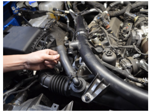
3. Disconnect the hose attached to the diverter valve.
