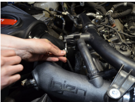
46. Reconnect the diverter valve harness.
