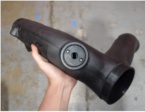
25. Place the temp sensor adapter onto the passenger side tube and secure using the provided M4 bolts.
