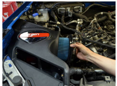
24. Install the twist lock filter on to the Injen air box. Once seated, rotate the filter a 1/4 turn in either direction so the filter can lock into place.
