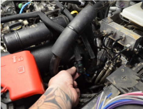
40. Reconnect both crankcase lines to the crankcase adapter.
