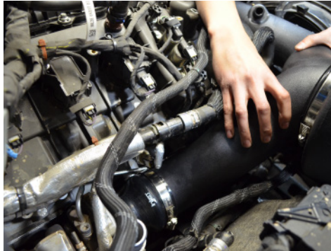
29. Install the passenger side intake tube. First, insert the tube to the hump hose then to the air filter.
