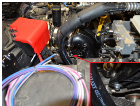
11. Remove the bolt securing the driver side intake tube to the engine.
