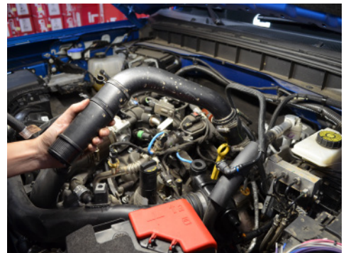
9. Loosen the clamp securing driver side charge pipe to the turbo then, remove the driver side charge pipe. You can access the clamp through the wheel well liner.
