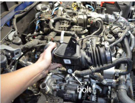
19. Remove the bolt securing the passenger side tube to the engine. Then detach the tube from the turbo. You can access the clamp through the wheel well liner.
