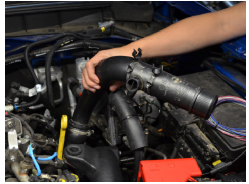
39. Reinstall the driver side charge pipe.
