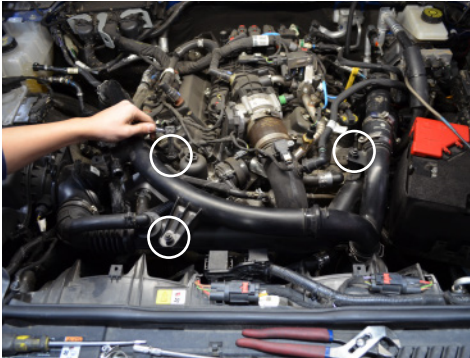
4. Remove the three bolts holding down the charge pipe.
