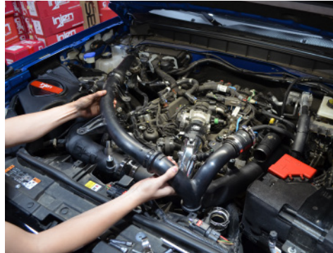
41. Reinstall the charge pipe.
