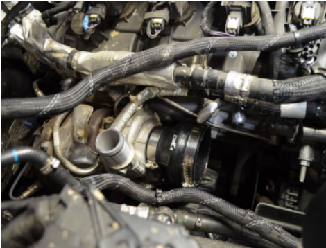
28. Attach the 2.00"-3.00" Stepping hump hose onto the passenger side turbo. Secure the hose with the provided clamps.
