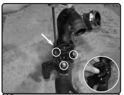
**12.** Loosen the 3 screws holding in the diverter valve using allen key. Carefully remove. Position new injen intercooler next to pipe for correct position.
