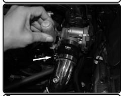
7. Tighten all clamps using 8mm nut driver.
