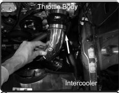
**6.** Now position the intercooler pipe into the hump hose on throttle body and secure. Adjust for proper fitment.
