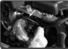
21. Secure the turbo side of the coupler and tighten using 8mm nut driver.
