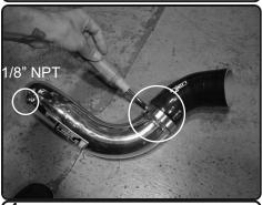
**4.** Secure the threadded fitting on intercooler tube if not using for auxilary boost/injection line with provided 1/8" NPT plug. Secure and tighten. Install the provided 2-1/2" elbow hose to the intake tube with clamps provided.
