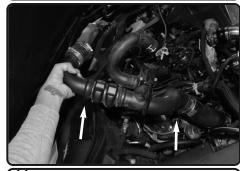
**11.** Now carefully lift up and remove the intercooler pipe out of vehicle.
