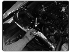
19. Install the hot side injen intercooler pipe into the vehicle. Position
