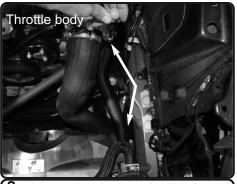
**2.** Loosen the clamp on the throttle body using 7mm nut driver. Loosen the clamp on the intercooler side also.
