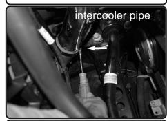
**20.** With soap water lubrication on the inside of the hump hose. This will allow for the elbow hose to slide on easier to intercooler. Tighten clamp using 8mm
