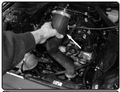
**7.** Carefully pull out the OEM rubber cold side intercooler hose out of vehicle.
