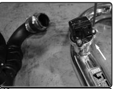
13. Secure the diverter valve to the injen intercooler pipe using allen key. Secure using original screws.
