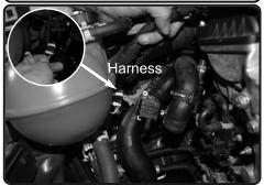
**9.** Disconnect the diverter valve harness. Pull line harness away from hot intercooler pipe.
