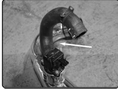
15. Secure the diverter line to the intercooler fitting.
