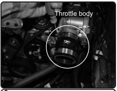
**3.** Install the provided 2-3/4" hump hose to the throttle body using provided clamps, tighten the clamp on throttle body only.
