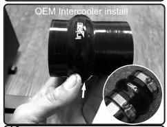
**16.** The 2.5" x 3.5"L hump hose seen above is for the installation with OEM intercooler only! **DO NOT CUT!**
