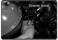
22. Re-connect the diverter valve harness.
