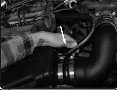
**15.** Install the provided 15mm hose to the airbox fitting.
