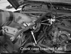
**6.** Remove the crank case line from the engine fitting.
