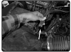
**3.** Pull back the crank case line from the stock intake box.
