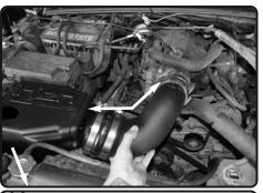
**14.** Insert the Injen intake tube into the hose on the throttle body and the hump hose on the Injen intake box assembly. Adjust the intake for best fitment and then secure all the clamps.
