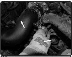
**17.** Reconnect the intake air temp sensor harness to the sensor.
