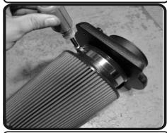
8. Secure the filter to the plenum.
