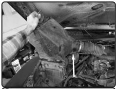
**5.** Firmly lift up and pull the factory air box assembly out of the engine bay.
