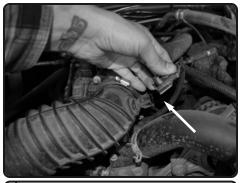
**4.** Disconnect the temperature sensor from stock intake system. Remove the temperature sensor from the intake tube.
