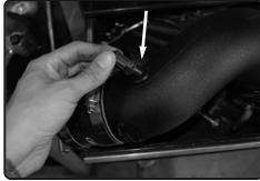
**12.** Place the grommet onto the 7/8" hole on the injen intake pipe and then insert the intake air temp sensor into the grommet
