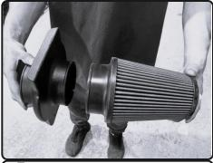
**7.** Place the filter onto the air box plenum
