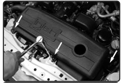
**33.** Secure and tighten all the screws using 10mm socket or wrench.
