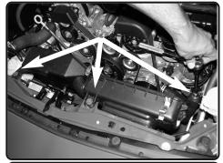
Loosen the 3 screws holding in the bottom half of the air box using 10mm socket and ratchet. Now lift up and remove the lower intake assembly from vehicle. Save for later install.
