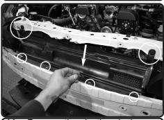
11. Remove the plastic splash guard from the front of vehicle, disconnect the push clips and remove.
