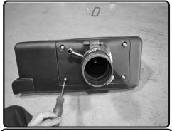
**28.** Secure and tighten using phillips screwdriver.
