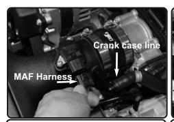
**37.** Secure and tighten all the screws using 10mm socket or wrench.
