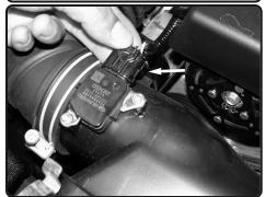
**5.** Disconnect MAF sensor harness and pull line away from air box.
