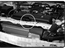
**38.** Secure the MAF sensor using provided M4 screws and tighten 2.5mm allen key.
