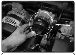
**31.** Position air box. Slide the hose on to the throttle body. Do not tighten .
