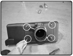
**27.** Install the plenum to the air box. Secure using phillips screws and rubberized washers.
