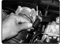
With pliers, pull back the crank case line from the intake fitting.
