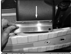
17. Install the ram scoop bracket to the ram scoop and the bumper support.
