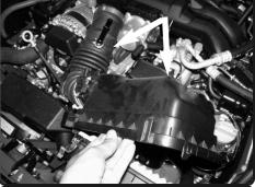
**6.** Unclip the upper part of the air box, remove the upper assembly including the intake tube from the vehicle.
