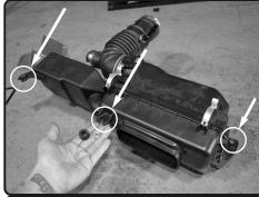
**20.** Remove the 3 grommets with crush spacer from stock air box. These will be used in new injen air box.
