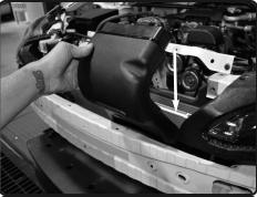
**16.** Install the ram scoop to the front of the vehicle between the bumper support and radiator.
