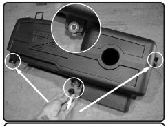
29 Now install the factory grommets with crush washer removed from the OEM air box (step 20)
