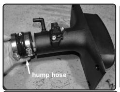
**25.** Install the 3" hump hose with clampsprovided to the intake plenum. Do not tighten.
