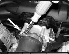
2. Loosen the clamp on the throttle body using 8mm nut driver.
