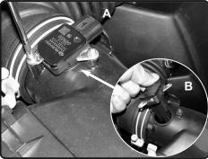
**8.** A)Loosen the 2 screws holding in the MAF sensor using the phillips screwdriver. B)Re-move the MAF sensor from the vehicle.
