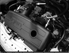
**30.** Push hump hose toward allowing for hose to slide back. Install the injen evolution intake assembly into vehicle.
