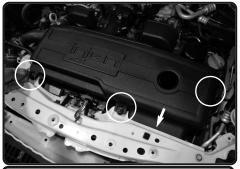
**32.** Make sure the injen box and the scoop are attached. Make sure the gasket is sandwiched between. Now secure the air box using the factory screws from step 7.
