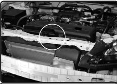
**36.** Secure the MAF sensor using provided M4 screws and tighten 2.5mm allen key.
