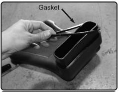
**15.** Install the provided gasket to the ram scoop.
