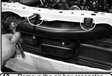
**10.** Remove the air box resonator by loosening the 2 bolts.
