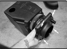
**10.** Insert the filter into the Injen air box. Use four M6X20 bolts and secure the Injen plenum to the Injen air box.
