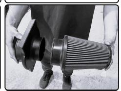
**7.** Place the filter onto the air box plenum
