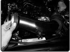
**3.** Remove the air duct from the throttle and air box. An intake air temp sensorwill need to be removed on the next step.
