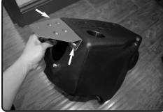
**9.** Place the Air Box Shield Air Director onto the opening of the air box. Secure the shield to the box with the two supplied M6X10 allen bolts. **Page 3 EVO5008**
