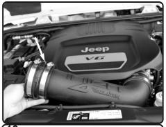
**13.** Place the 4.00" hump hose and two #64 clamps onto the big end of the Injen intake tube. Make sure you slide the hose all the way over onto to tube.
