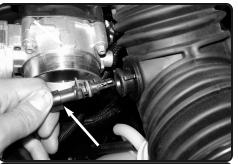
**4.** Locate the intake air temp sensor underneath the factory air duct from figure 7. Disconnect the harness and twist the IAT sensor to remove the sensor from the air duct.
