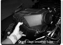
**5.** Disconnect the crank case breather tube. Then firmly lift up and pull the factory air box assembly out of the engine bay.
