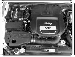
**15.** Connect the crank case vent tube to the port on the Injen air box assembly.
