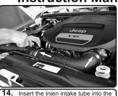
**14.** Insert the Injen intake tube into the hose on the throttle body and the hump hose on the Injen intake box assembly. Adjust the intake for best fitment and then secure all the clamps.
