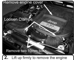
cover. Continue to loosen the two clamps from the throttle body and air duct. Then remove the two 10mm bolts pictured.
