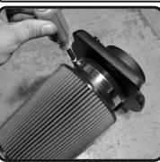
**8.** Then secure the filter to the plenum.
