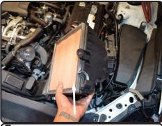
7. Lift up and remove the lower part of air box out of vehicle. Leave the front OEM ram scoop in vehicle.
