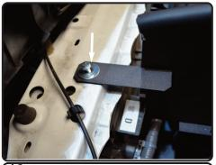
**16.** Place tab over the thredded insert. Secure using provided M6 hex screw and fender washer.
