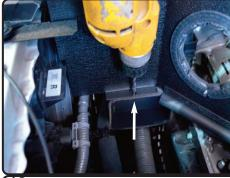
**18.** Drill hole to 1/4" on the OEM ram scoop.
