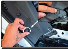
**12.** Push down on the clips on the radiator cover, remove clips and guard for installation of heatshield.
