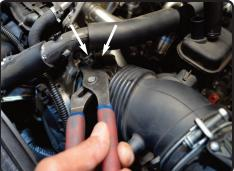
**4.** With pliers or channel locks carefully de-press the large clamp on the throttle body. Pull back the intake tube from the throttle body.
