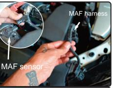
**2.** Disconnect the MAF sensor harness and pull harness cable from the air box.
