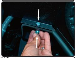
**19.** Secure using provided M6 screw and nut.
