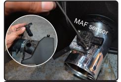
**11.** Remove the MAF sensor using phillips screwdriver. Install into the new intake tube and secure using provided M4 button head screws.
