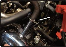
**22.** Re-connect the crankcase line to the 5/8" fitting on the intake tube. Secure using the OEM clamp.
