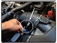
**75.** Pull back the vacuum line away from the intake tube.
