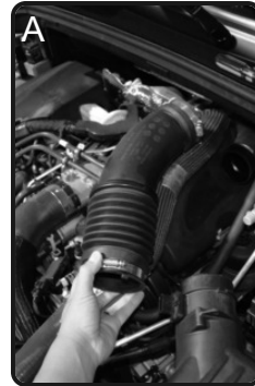
3. Figure A: Remove the O.E. intake tube. Figure B: Remove the upper O.E. air box assembly.
