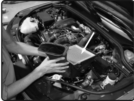
4. Firmly lift up on the O.E. lower air box assembly and remove from the engine bay.
