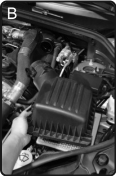
3. Figure A: Remove the O.E. intake tube. Figure B: Remove the upper O.E. air box assembly.
