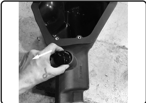
9. Install the Filter Minder plug into the Filter Minder pod on the lower air box assembly
