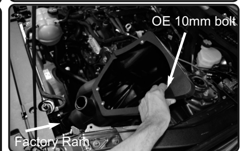
12. Drop the Injen lower air box assembly into the factory air box location. The front ram air should just slide into the Injen air box, Then secure the lower box to the chassis with the original 10mm bolt.
