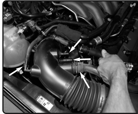
2. Disconnect the three vacuum lines and sound tube from the factory intake air duct.
