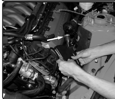
6. Disconnect the sound tube resonator box.
