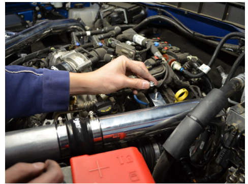
51. Secure the tertiary hot side intercooler pipe with the provided M6 nut and washer.
