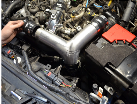
41. Attach the 2.25" hump hose to both ends of the cast Y-Pipe. Secure using the provided clamps.
