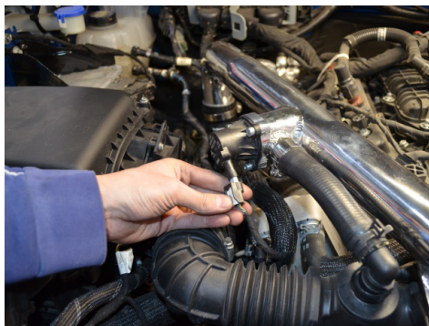
47. Reconnect the diverter valve harness.
