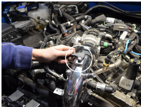
32. Install the OEM pressure sensor onto the Intercooler pipe. Secure with the provided M6 bolt.
