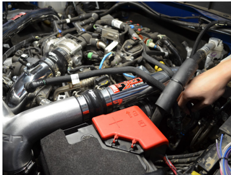
53. Reconnect both crankcase lines to the intake tube.
