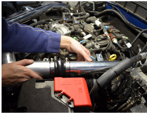
50. Install the tertiary hot side intercooler pipe. Secure using the provided clamps.
