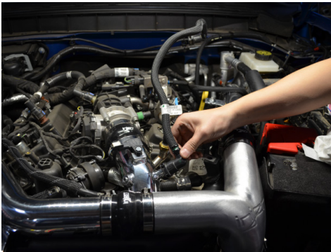
52. Reconnect the crankcase line to the cold side intercooler pipe. Reconnect the pressure sensor harness.
