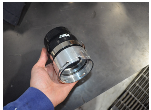
36. Attach the 2.75" hump hose to the intercooler adapter. Secure using the provided clamps.
