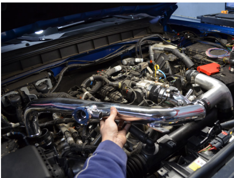
43. Install the secondary hot side tube.
