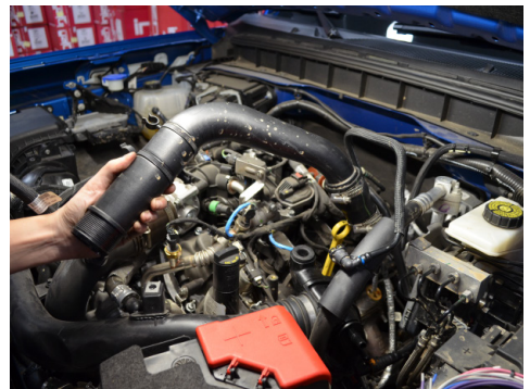
9. Remove the driver side intercooler pipe.
