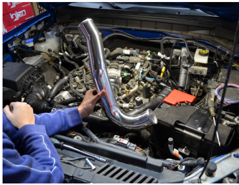
38. Install the primary hot side intercooler pipe. NOTE: Make sure this pipe is completely bottomed out on the adapter in fig. 39
