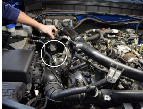
5. Detach the hose connecting the intercooler pipe to the passenger side turbo.
