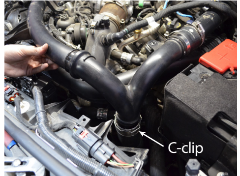
6. Pull back the intercooler pipe C-clip and then lift up the intercooler pipe.
