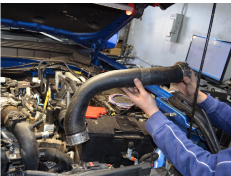
22. Remove the hot side intercooler hose.
