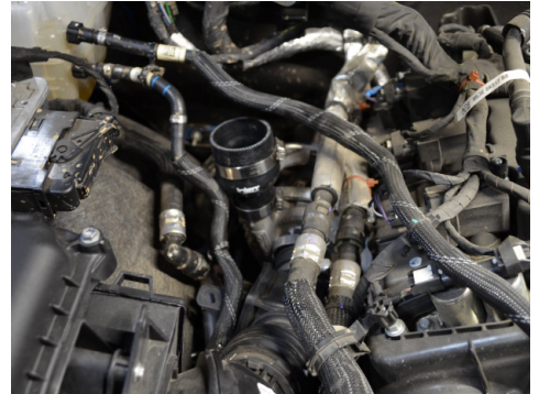
42. Attach the 1.50"-2.25" stepping hump hose to the passenger side turbo outlet. Secure using the provided clamps.
