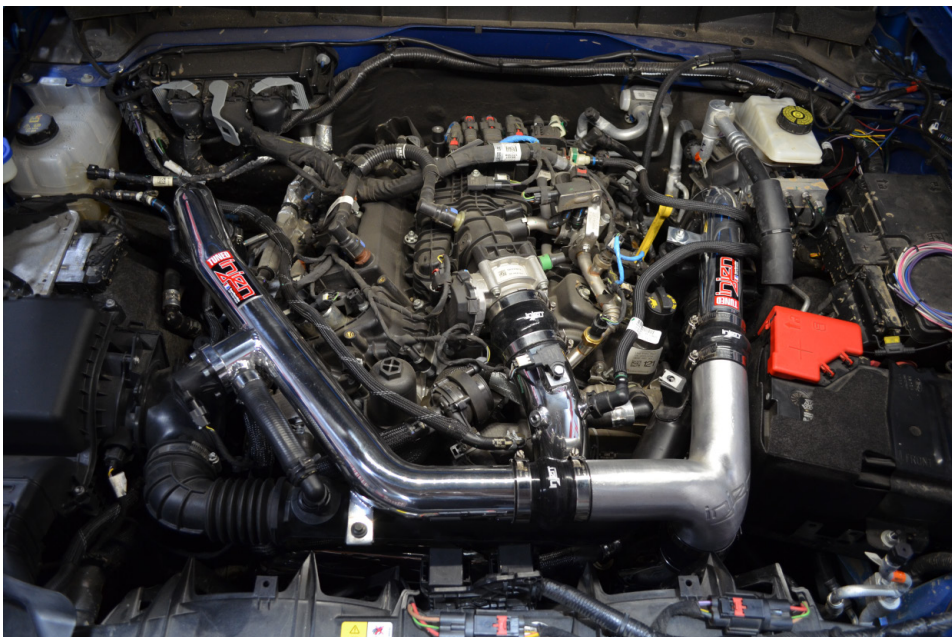
52. Reconnect the crankcase line to the cold side intercooler pipe. Reconnect the pressure sensor harness.
