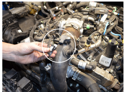
12. Disconnect the pressure sensor harness.
