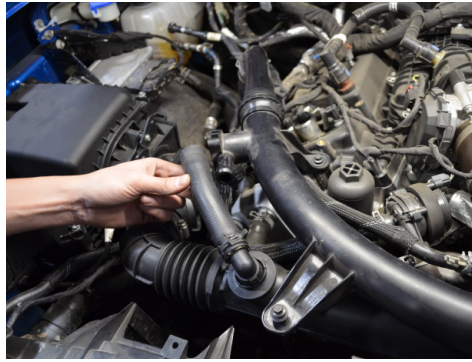
2. Disconnect the hose attached to the diverter valve.
