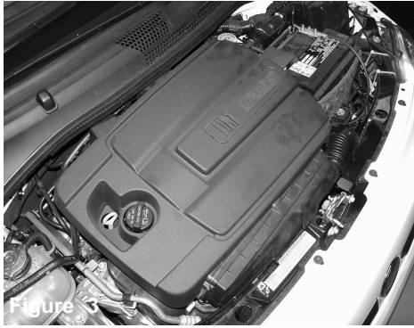
Figure 4 Lift up the engine cover, and remove.
