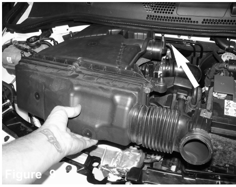
Figure 9 Pull out the complete air box assembly. Make sure the coolant line is apart from the back of the air box.
