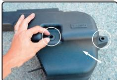
**10.** Install the remaining 2 grommets to the holes on bottom of injen air box and secure.
