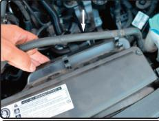
7. Loosen and pull back the coolant line from the OEM ram-scoop.
