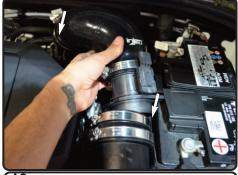
**19.** Install the MAF with molded turbo hose into position. Do not tighten.
