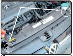
**6.** Loosen the 2 screws holding in the front OEM ram-scoop using T25 torx bit. Save screws for later install. Push clips down out of the radiator support.
