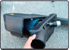
11. Install the plenum assembly into the air box.
