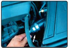
**23.** Connect the OEM air pump fitting to the machined fitting on intake plenum. If not equipped with air pump, use supplied air pump cap.
