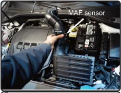
**5.** Disconnect the MAF sensor. Now lift up OEM intake air box assembly out of vehicle.
