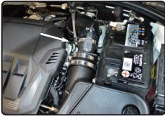
**22.** Adjust the MAF sensor harness for proper fitment and not kinking.
