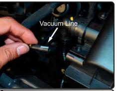
**2.** Remove small vacuum line from the factory airbox.
