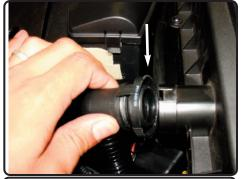
**3.** If equipped with air pump, pinch the harness on smog pump and pull away from air box.
