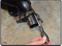
**16.** Loosen and remove the 2 T25 torx screws from the air box. Remove the MAF sensor from the air box.
