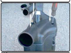
**12.** Secure using provided 3 M6x20mm phillips screw with 3 rubberized washer.
