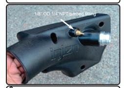
**9.** Install and secure the 1/8" NPT 1/4" barbed fitting to the plenum insert and tighten.
