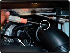
**4.** With 7mm nut driver, loosen the clamp on turbo housing.
