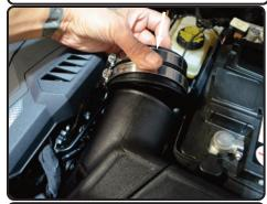
17. Install the provided Step hose with clamps to the plenum on the air box.
