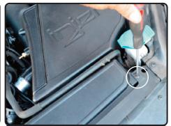
**15.** Now secure the injen driver Ram scoop using the factory screws from step 6
