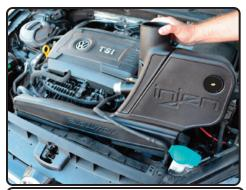
**13.** Install the intake assembly into the vehicle. Position to factory holes. Make sure the intake assembly seats in studs.
