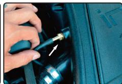
**24.** Now connect the vacuum line to the 1/8" NPT 1/4" barbed fitting.
