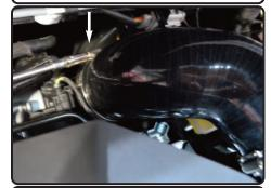
**21.** Adjust for proper fitment. Tighten all clamps using 8mm nut driver.
