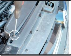
**14.** Now secure the passenger injen Ram scoop using the factory screws from step 6.
