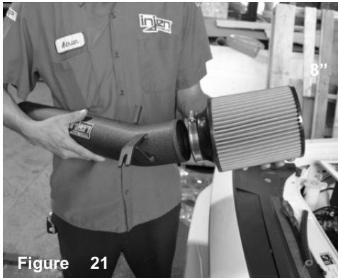
Figure 21 Place the filter onto the bracket end of the secondary tube
