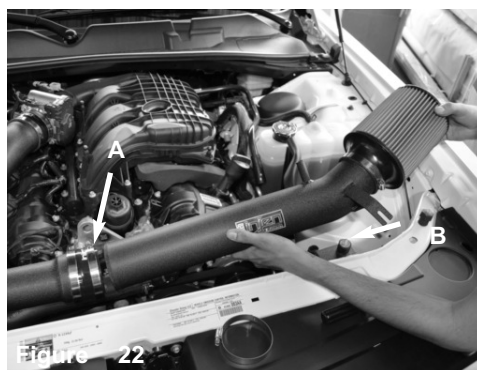
Figure 22 (A) Position the other end of the secondary tube into the primary tube from figure 15 (B) Also, Align the Bracket on the secondary tube to the vibramount on the radiator support from figure 20.
