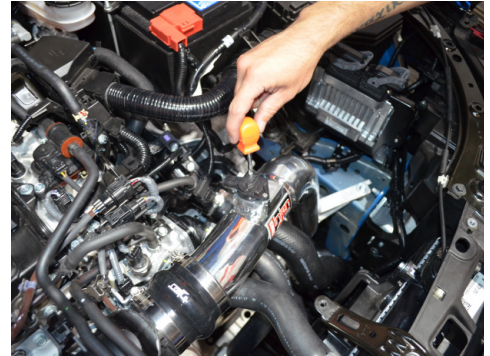
18. Install the MAF sensor onto the intake tube and secure using the OEM bolts.
