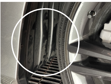
22. Due to the large diameter of the intake, the intake tube will push on the wheel well liner. Turn the wheel in both directions to ensure the tire does not touch the wheel well liner.
