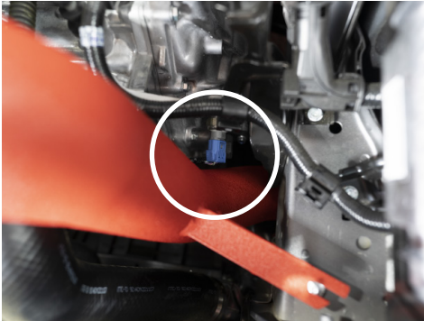
16. Ensure there is a minimum of .500" clearance between the intake and the transmission sensor. Adjust the intake for proper clearance.
