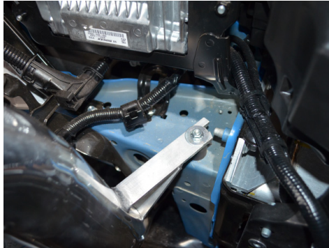
17. Secure the intake tube bracket with the provided M6 bolt and washer. Resecure the ECU to its factory position from figure 11.
