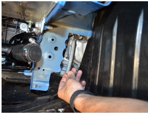
14. Attach the vinyl trim to the chassis. This will protect the tube from hitting the chassis.
