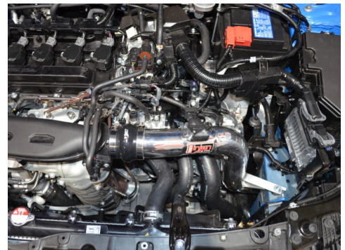
21. Adjust the intake tube for best fitment and then ensure all nuts, bolts, and clamps are properly secured. Reinstall the front bumper.
