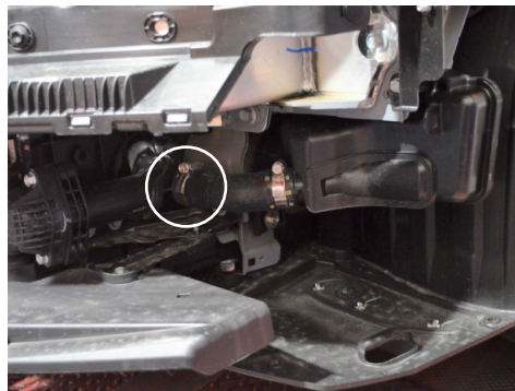
8. Loosen the clamp securing the intercooler pipe resonator to the intercooler pipe.
