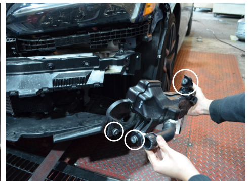
9. Remove the three bolts securing the intercooler pipe resonator, then remove the resonator.
