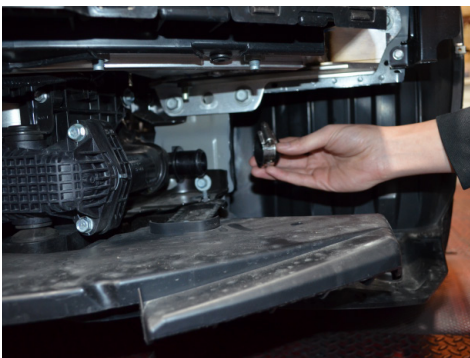
10. Use the reinforced cap and #20 clamp to cap of the port on the intercooler piping.
