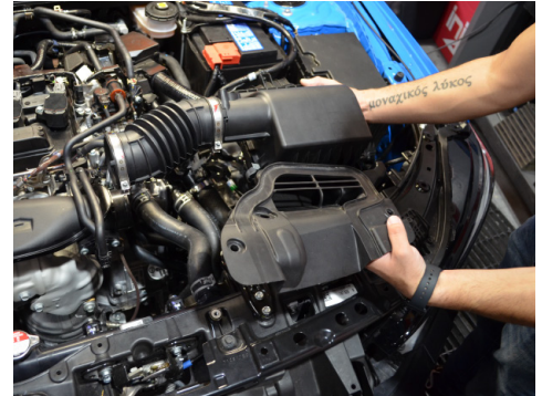
6. Remove the OEM intake system by firmly lifting up.
