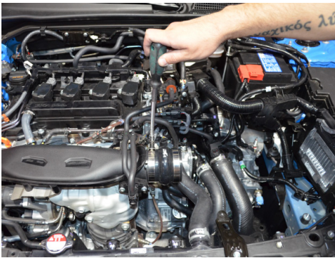
13. Attach the 2.625"-2.75" stepping hump hose to the turbo inlet. Secure the turbo side clamp only for now.
