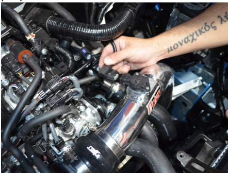
19. Reconnect the MAF sensor harness.
