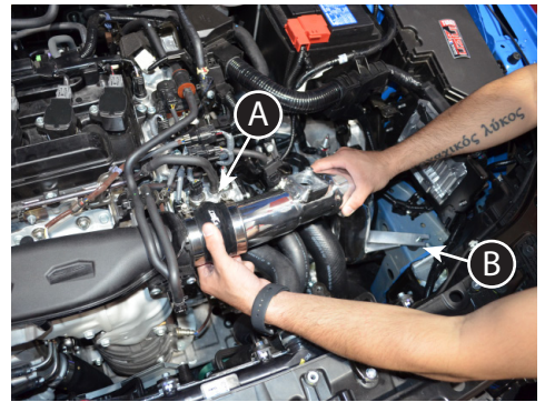
15. (A) Install the injen intake tube into the stepping hump hose. (B) Line up the bracket to the M6 vibra mount.
