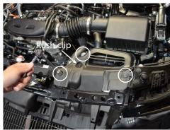
front air scoop, then remove the push clip with a prying tool.
