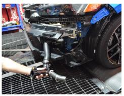
12. Remove the bottom half of the cold side intercooler pipe.
