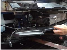
35. Secure the intercooler adapter to the inlet on the intercooler using the the OEM bolts.
