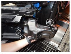
9. Remove the three bolts securing the intercooler pipe resonator, then remove the resonator.
