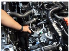
10. Loosen the clamp securing the rubber intercooler hose to the top half of the cold side intercooler pipe, then detach the hose.
