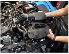
6. Remove the OEM intake system by firmly lifting up.
