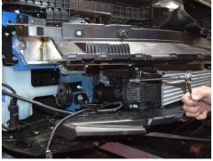
20. Remove the two bolts securing the intercooler pipe to the intercooler.
