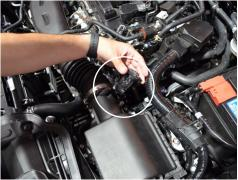
2. Remove the two bolts securing the MAF 3. Remove the three bolts securing the sensor then remove the sensor.
