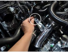
25. Install the primary cold side intercooler 26. Secure the intercooler pipe bracket to the M6 vibra mount with the provided M6 the provided M6 bolt. nut and washer.
