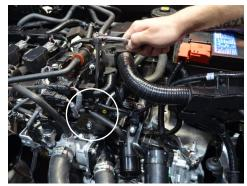
13. Remove the two bolts securing the intercooler pipe bracket to the engine.
