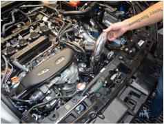
38. Install the hot side intercooler pipe. Insert the pipe into the bottom hose then into the top step hose.
