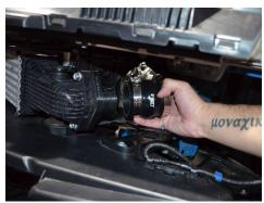
32. Install the 2.25" hump hose onto the intercooler adapter. Only secure the clamp intercooler pipe. Insert the pipe into the on the intercooler adapter.
