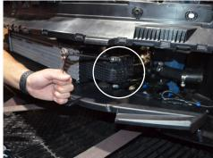
11. Remove the two bolts securing the cold side intercooler pipe to the intercooler.
