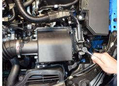
4. Remove the bolt securing the side of the airbox to the chassis.
