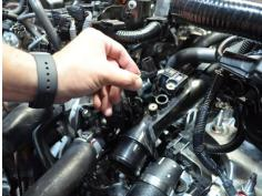
17. Carefully remove the pressure and temp sensor from the intercooler pipe.
