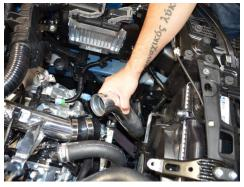
33. Install the secondary cold side bottom hose then into the top hose.
