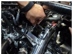
29. Reconnect the vacuum line to the vacuum fitting on the intercooler pipe.
