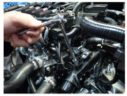
16. Disconnect the pressure and temp sensor harness, then remove the bolts securing the sensors.
