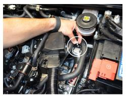
27. Secure the coolant line bracket with
