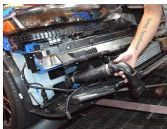
21. Remove the intercooler pipe from the vehicle.
