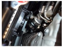
37. Install the 1.875"-2.25" hose onto the turbo. Only secure the clamp on the turbo.
