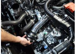
28. Install the 2.25" hump hose with clamps onto the intercooler pipe. Leave the clamps loose.
