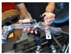
24. Install the pressure and temp sensor onto the injen cold side primary intercooler pipe. Secure both with the OEM bolts.
