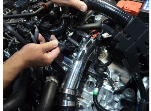
30. Reconnect the temp and pressure sensor harness.
