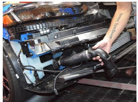
21. Remove the intercooler pipe from the vehicle.
