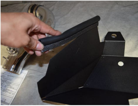
13. Install the 10" bulb trim onto the top edge of the heatshield. Trim the bulb trim if necessary.
