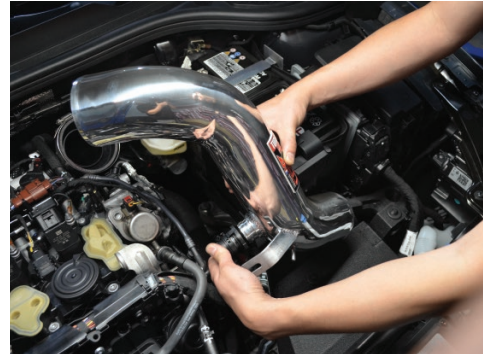
18. Connect the secondary air injection tube to the injen intake tube.
