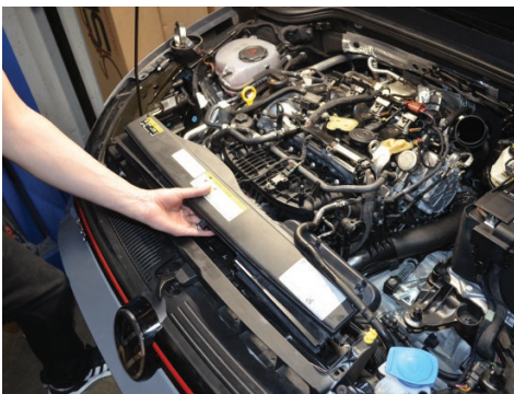
10. Re install the front scoop and secure using the two OEM screws.
