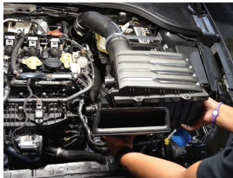
8. Remove the intake assembly from the engine bay. Note: Grommets are attached to the air box, apply lubricant if necessary.
