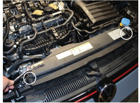
6. Remove the two screws holding the front air scoop.
