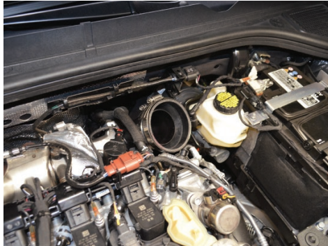
17. Install the step hose onto the turbo inlet. Attach both clamps onto the hose and secure the turbo side clamp.
