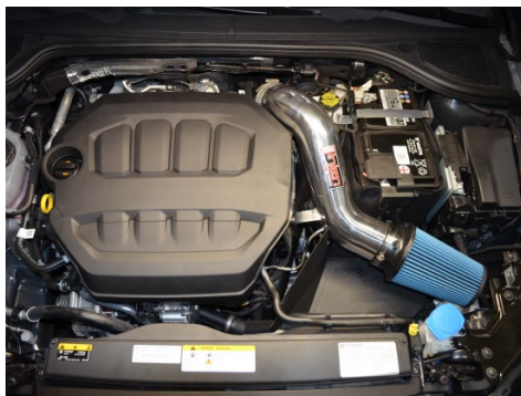
24. Ensure that all bolts, clamps and hoses are properly secured. Re install the engine cover.
