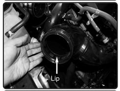
**17.** Now install the 4" elbow with provided clamps to the drivers side large turbo inlet. Position like image above. Leave clamps loose for now.
