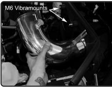
**19.** Install two vibramount to the threaded inserts on heat shield. Install the large intake pipe, make sure the 3.5" side goes through hea shield. Position the bracket to the vibramount and tube to 4" elbow. Do not tighten.
