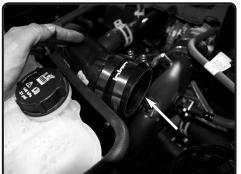
**18.** Install the 3" straight hose with provided clamps to the passengers side turbo inlet. Tighten the clamp on housing only using 8mm nut driver.
