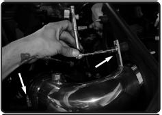
**21.** Use a 10mm socket and ratchet to secure the bracket to the vibramount with a provided M6 nut and fender washer. Tighten clamps using 8mm nut driver.
