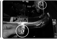
24. Secure the brackets using provided M6 nuts and fender washers.
