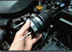
**10.** Install the provided step hose with clamps provided to the turbo housing.
