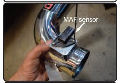
**9.** Install the MAF sensor into the intake tube and secure using M4 button head screws. Tighten using 2.5mm allen key.
