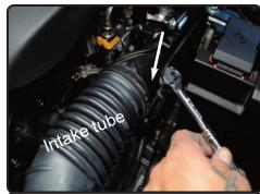
**4.** Loosen the clamp on the OEM intake tube using 10mm socket or nut driver.
