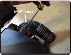
**8.** Remove the 2 screws holding in the MAF sensor.
