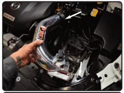
**15.** Install the intake tube and position to the step hose and bracket to the vibrmount.
