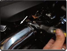
**16.** Adjust and tighten the clamp on the intake tube usng 8mm nut driver.
