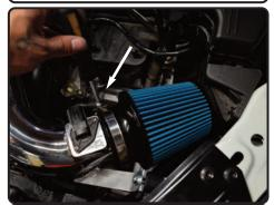
**17.** Install the filter to the intake tube and tighten using 8mm nut driver.
