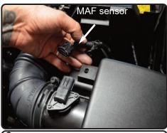
**3.** Disconnect the MAF sensor, and pull back the harness away from the air box.
