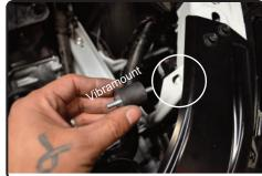
**12.** Locate the slot on the frame above headlight and radiator support. This is where the vibramount will go.
