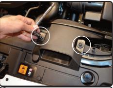
**2.** Remove the 2 screws holding in the top of the factory ram scoop. Remove the 2 screws using 10mm socket or wrench.
