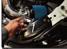
**19.** Adjust the intake for fitment and tighten the bracket using 10mm socket or wrench.
