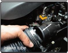
**5.** Pull back the intake tube away from the turbo housing.
