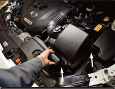
**6.** Carefully lift up the air box assembly.
