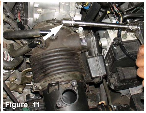
Figure 11 Loosen the clamp on the throttle body air hose as shown above.
