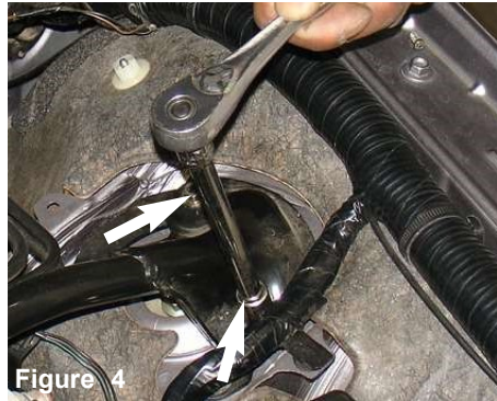
Figure 4 OPTIONAL: Loosen and remove the two 12mm nuts located on the each strut tower mount. Once you have removed all four 12mm nuts, continue to removed the strut tower bar.
