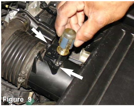
Figure 9 Unscrew and remove the two screws that fastens the mass air flow sensor to the sensor housing.
