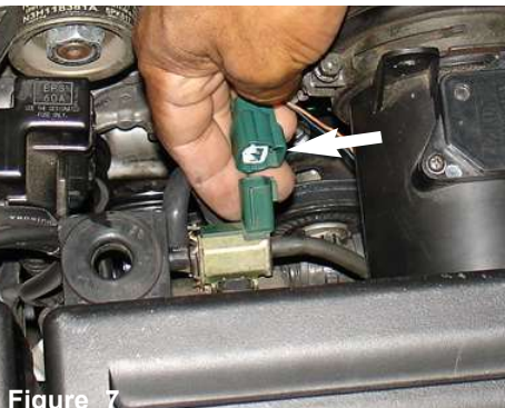
Figure 7 Depress the tab on the green electrical clip and pull the clip from the vacuum switching valve. Note: on automatic transmissions, skip step and go to figure 8.
