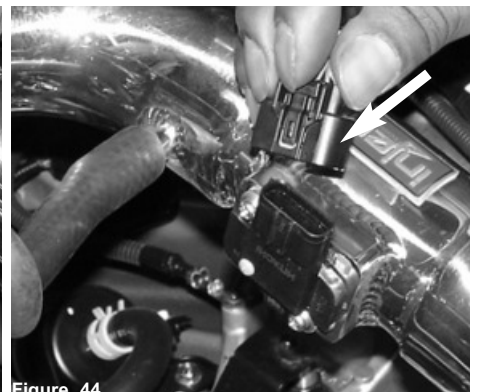
Figure 44 The electrical harness is pressed over the MAFS until it you hear them snap together.
