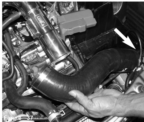
Figure 37 The silicone intake is inserted into the front bumper opening.
