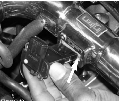
Figure 42 The MAFS is inserted into the sensor adapter as shown above.
