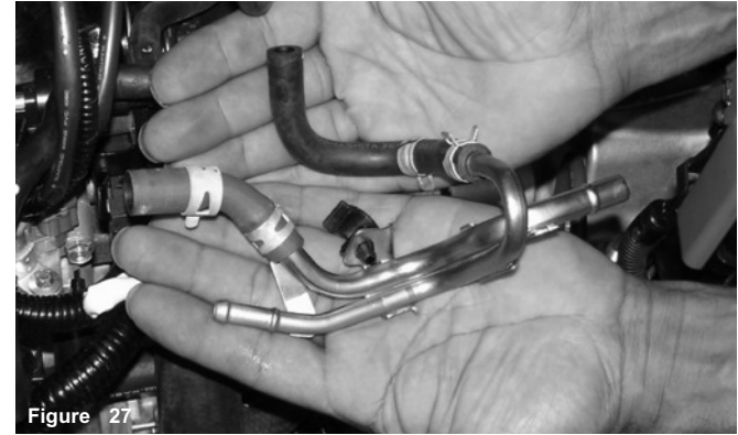
Figure 25 The lower coolant line is pulled from the PCV hard line.
