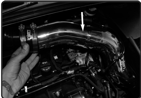
20. Install the intake and position the bracket to the stand off stud.
