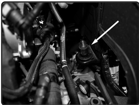
16. Install the M6 stand off stud to the grommet of OEM airbox mounting bracket.
