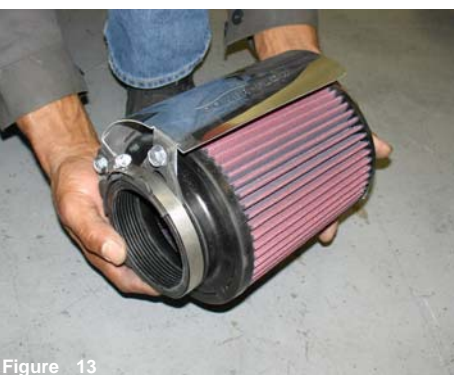
Figure 13 Filter and heat shield assembly is now complete.
