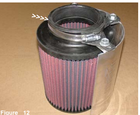
Figure 12 Adjust the clamp so that it sits between the filter beads located on the filter neck.
