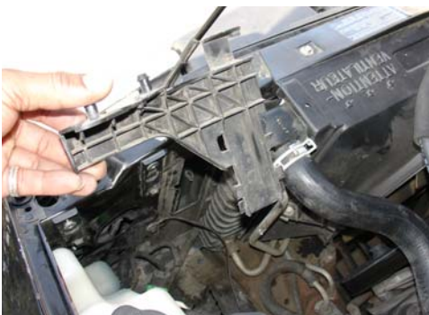
Retract plastic pins in order to allow the bracket to become loose.
