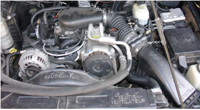
Loosen all clamps from the throttle body plastic air inlet to the mass air flow sensor.
