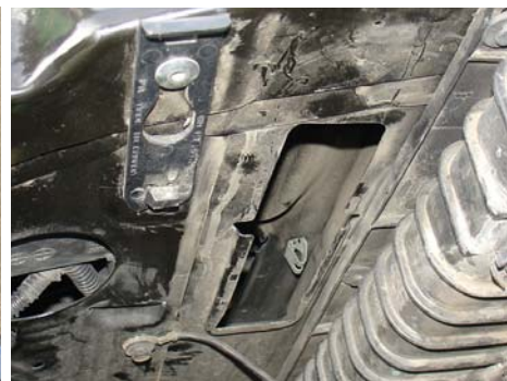
More clearance has been made for the new larger filter.
