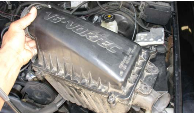
Pull the air intake box out from the grommets and remove the air intake box.
