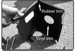
**10.** Attach the rubber trim to the top of heatshield. *Using pliers notch corners for easier install.*
