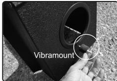
**11.** Attach the M6 vibramount to the heat-shield, secure and tighten.
