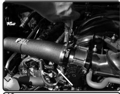
**19.** Position the tube for best fit. Tighten the clamp on the throttle body using 8mm nut driver.
