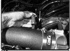
**18.** Install the crankcase line to the fitting on the intake tube. Secure using the OEM clamp.
