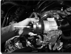
**15.** Install the 3-1/4" straight hose with clamps to the throttle body. Tighten clamp on throttle body only.
