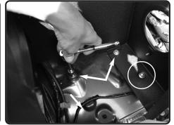
14. Now secure the vibramount with provided M8 nut and small washer. Secure the 2 remaining holes on heatshield with provided M8 screws and small washers. Secure and tighten.
