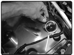
**12.** Install the provided M8 vibramount to the fitting to the OEM airbox thredded insert location.
