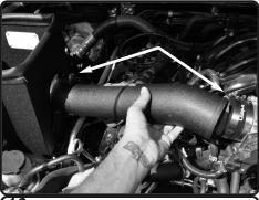
**16.** Install the intake tube into the vehicle. Position the tube to the throttle body and bracket to the vibramount.
