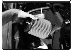
**20.** Install the filter and position to intake tube. Secure the filter and tighten clamp using 8mm nut driver.
