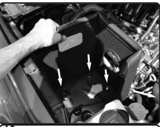
**13.** Install the heat shield and position the tab with dimple-die to the vibamount.
