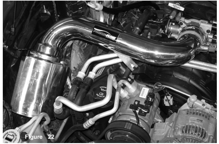
Figure 22 Periodically, Check the fitment of the intake system. Check all lines, clamps, bolts and filter parts for any possible misalignment. The filter should also be checked and cleaned every 5000 to 7500 miles. Hydro-shields are also sold on-line that will help extend the life of your filter.
