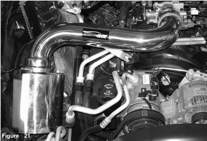
Figure 21 Align the entire intake assembly for the best possible fit. Once the intake, filter and heat shield have been adjusted and cleared from any moving parts, continue to tighten all nuts, bolts and clamps.
