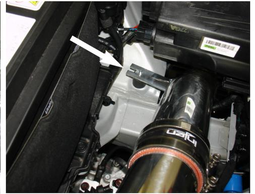
**27.** Secure both brackets with the provided M6 nut and washer.
