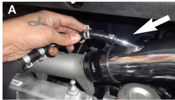
14. **Figure A:** Connect the crank case breather line to the 0.5" nipple on the intake pipe. **Figure B:** Connect the recirculating diverter valve hose onto the 1.0" nipple onto the intake pipe
