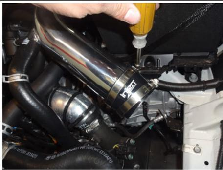
20. Place the 3.0" straight hose and two clamps onto the intake tube. Only secure the clamp on the intake side for now.
