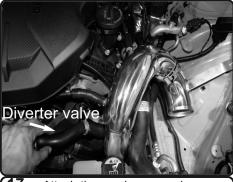
17. Attach the crank case and vacuum line to the intake tube. Attach the diverter line to the large fitting on intake tube.
