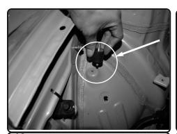
**12.** Install the provided vibramount to the original air box mounting location. Insert on passenger side. Secure and tighten.
