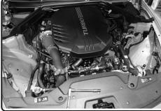
**11.** Both stock intakes removed from vehicles.
