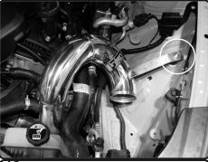
**18.** Secure the bracket on driver side using provided fender washer and nut. Position intake for the best fit and tighten clamps using 8mm nut driver.
