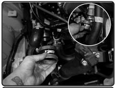
**14.** Install the provided 2-1/4" straight hose to the turbo on both sides with clamps. Tighten clamp on turbo side only using 8mm nut driver.
