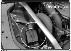
**21.** Install the air filter to the passenger side and tighten using 8mm nut driver. Readjust if necessary for best fit.
