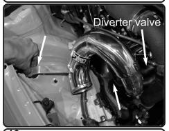
**19.** Install the passenger side tube and po-sition the bracket to the vibramount and turbo. Attach the diverter line to the large fitting on intake tube. Do not tighten.
