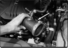
**9.** Remove the intake tube from both sides.
