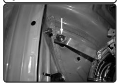
**20.** Secure the bracket on passenger side using provided fender washer and nut. Position intake for the best fit and tighten clamps using 8mm nut driver.
