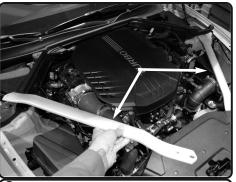
**2.** Loosen and remove the 2 strut braces on passenger and driver side.
