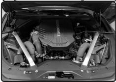
**23.** Re-install the strut braces to the vehicle.
