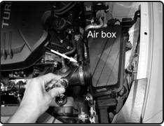
**3.** Loosen clamp on air box on both sides using 10mm socket or nut driver.
