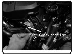
**6.** On driver side only, loosen clamp and pull back the crank case line from engine.
