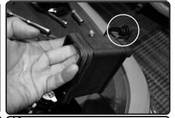
**10.** Loosen the 2 bolts holding in the plastic air box inlet using 10mm socket or wrench and remove on both sides.
