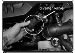
**8.** On both sides, loosen clamp and pull back the diverter valve.
