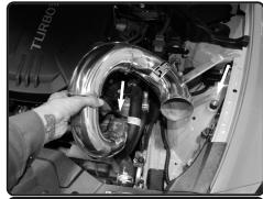
**15.** Install the Driver side tube and position the bracket to the vibramount and turbo. Do not tighten yet.
