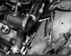
7. Loosen the clamp on the turbo using 10mm socket or nut driver on both sides.
