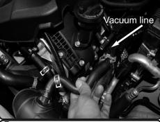
**5.** On driver side only, Loosen clamp and pull back vacuum line from engine.
