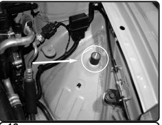
**13.** Install the provided vibramount to the original air box mounting location. Insert on driver side. Secure and tighten.
