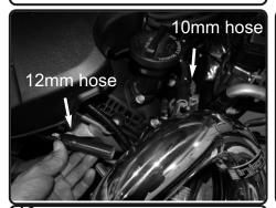
**16.** Install the provided 12mm hose to the crank case fitting and 10mm hose to the vacuum fitting. If long, cut to desired length.
