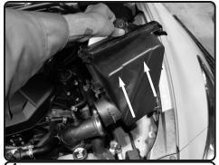
**4.** Carefully lift up and remove the air box on both sides.
