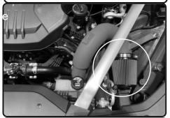
**22.** Install the air filter to the driver side and tighten using 8mm nut driver. Re-adjust if necessary for best fit.
