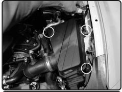
7. Loosen the 3 bolts holding in the OEM air box for both sides usin 10 mm socket with ratchet.
