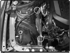
Locate the 2 threaded studs in the engine compartment, this will be used for the heat shield.
