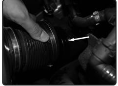
7. Loosen the clamp on air box and pull back the intake tube.
