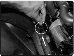
**4.** Carefully lift up and remove the entire stock air box assembly.
