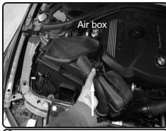
**3.** Now lift up and pull the entire air box assembly out of the vehicle.
