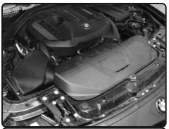
**1.** Stock intake system shown. Lift up and remove the front radiator cover.
