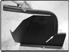
**6.** Install rubber trim to the top of the heatshield. Notch corner for easier installation.
