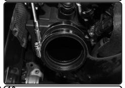
**10.** Tighten the clamp on the turbo side only using 8mm nut driver.
