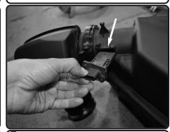
**7.** Remove the 2 screws holding in the MAF sensor using T25 torx bit.
