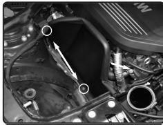
**15.** Push and secure and make sure the grommets are seated and secured to the studs.
