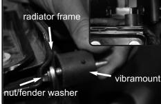
11. Install the provided M6 vibramount to the radiator support. Use provided M6 nut and fender washer to secure the backside of the vibramount.
