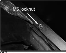
17. Secure and tighten the bottom of the heatshield using provided M6 lock nut. Secure and tighten using 10mm socket or wrench.
