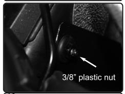
**16.** Secure the tab on heatshield near firewall using the provided 3/8" plastic nut. Secure and tighten.
