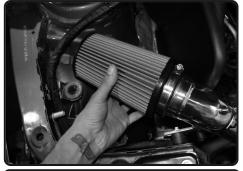
**22.** Install the filter to the intake tube. Secure and tighten the filter using 8mm nut driver.
