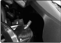
**23.** Re-install the radiator cover. **Note:** fitting on intake tube is for grommet on radiator cover to seat and secure.
