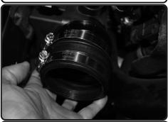
**9.** Install the provided step hose with clamps to the turbo.
