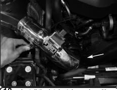
**18.** Install the intake tube and position the bracket to the vibramount.
