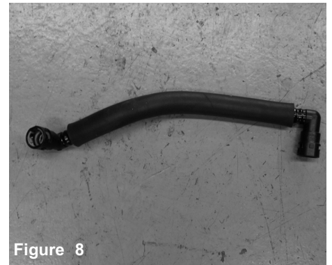
Figure 8 The entire crankcase vacuum hard line is now removed.
