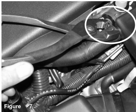
Figure 7 Depress the tension clamp on the crank case breather hose and pull it away from the crank case vent box.
