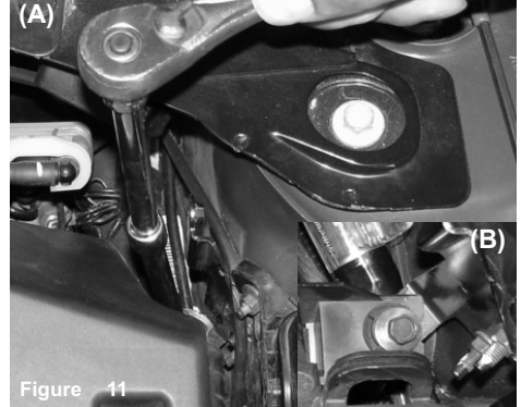
Figure 11 A 10mm socket and ratchet is used to remove an m8 bolt (A). The m8 bolt is located just behind the top air box on the right hand side (B).
