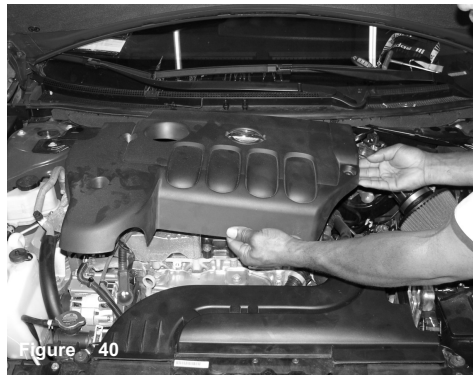
Figure 40 The engine cover is placed over the engine to its original position.
