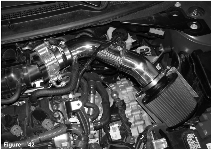
Figure 42 adjust the entire intake for the best possible fit. Once you have made proper clearance through-out the intake and heat shield, continue to tighten all nuts, bolts and clamps.
