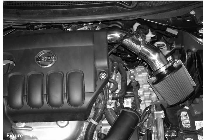
Figure 43 Periodically, check the fitment of the intake and heat shield. Normal wear and tear may causes shifting of the intake that may cause damage to the intake. Failure to perform monthly preventative maintenance will void the warranty of this intake system.
