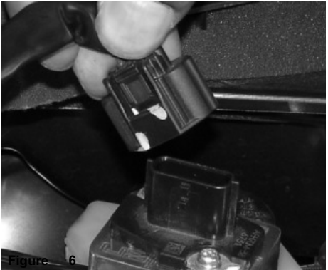
Figure 6 Press the clip on the harness connector and pull the electrical harness from the mass air flow sensor.
