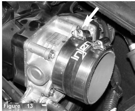
Figure 13 Press the 2 3/4" straight hose over the throttle body and use two power bands. The power band on the throttle body is tightened at this point.
