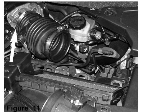
Figure 11 The upper air box is now separated from the lower air box cleaner.
