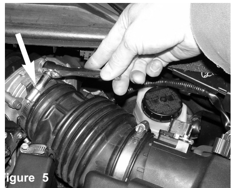
Figure 5 Loosen the clamp located over the throttle body.
