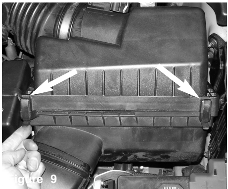
Figure 9 Unlatch the two metal clips shown above.
