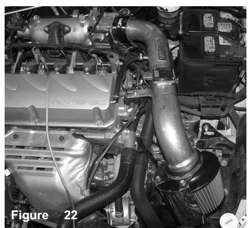
Figure 19 Place the filter and heat shield assembly on to the end of the intake pipe. Use a 8mm nut driver and tighten the clamp on the filter
