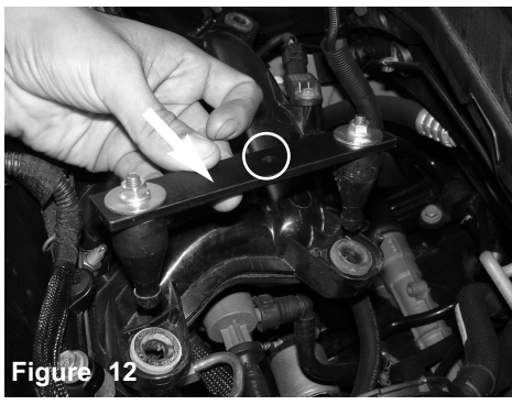
Figure 13 Secure and make sure the bracket is seated in grommets.
