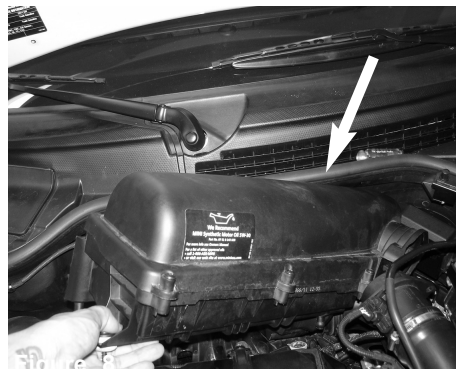
Figure 8 Now lift up and remove the stock air box from the vehicle, this may require some force.
