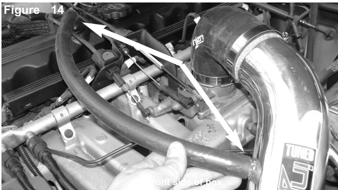
Intall the 15mm hose to the engine and the fitting on the intake tube.
