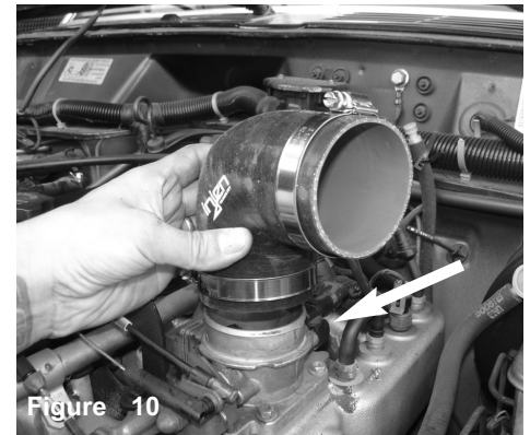
Figure 10 Now with the shortest side of the elbow hose, install to the throttle body with clamps provided.
