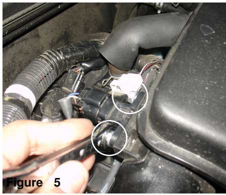
Figure 5 With 10mm wrench, loosen the 2 screws holding in the vacuum sensor. Note : this is not a part of the intake system nor will be used with Injen set up.
