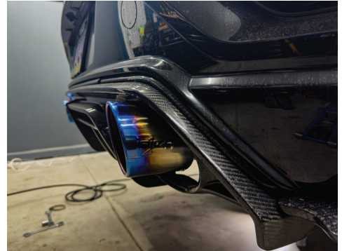
6. Adjust the exhaust tips to the desired location then secure the clamps.
