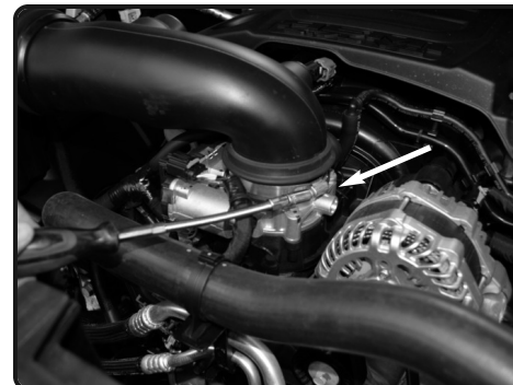
3. Loosen the clamp on the throttle body using 8mm nut driver.
