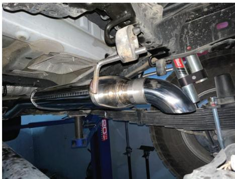
11. Secure the HT-Rear pipe to the muffer section using the 76mm clamps. Once complete, ensure all bolts and clamps are properly secured.
