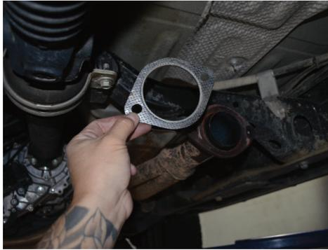
5. Install the provided exhaust gasket.
