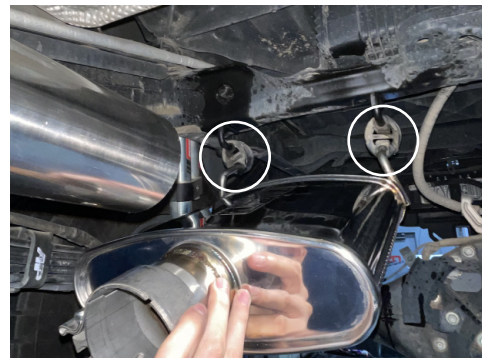
9. Insert the muffer hangers into the rubber insulators.
