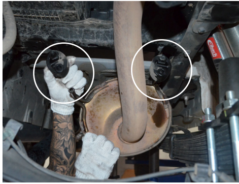
2. Detach the three muffer hangers from the rubber insulators.
