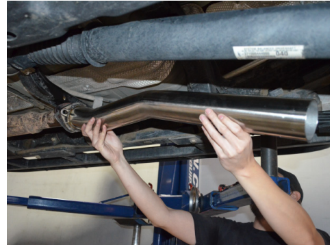
6. Attach the Injen front pipe to the OEM exhaust pipe.
