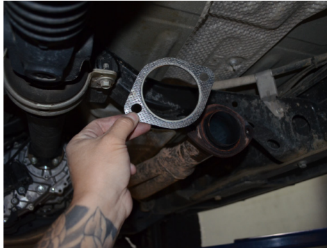
5. Install the provided exhaust gasket.
