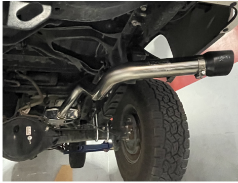
14. Ensure all bolts and clamps are properly secured.
