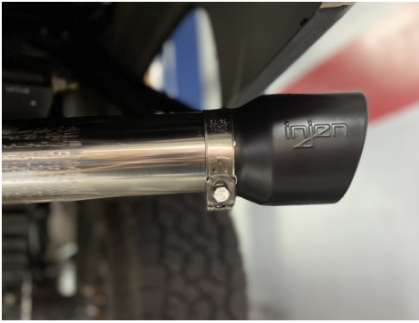
13. Attach the exhaust tip to the rear pipe. Adjust the exhaust tip for best fitment.
