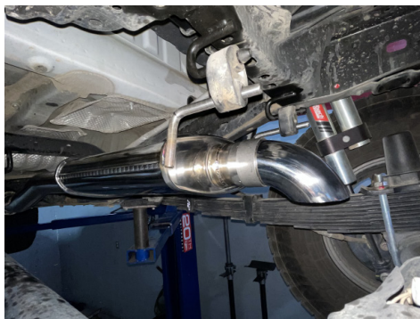
11. ALTERNATIVE HIGH TUCK OPTION : Secure the HT-Rear pipe to the muffer section using the 76mm clamps.
