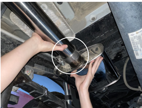
10. Secure the muffer section to the front pipe with the provided 76mm clamps.
