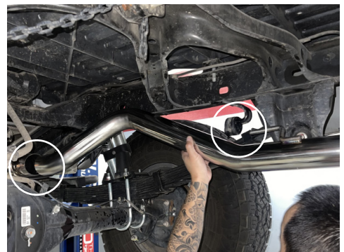
12. Insert the rear pipe hanger into the rubber insulator, then secure the pipe to the muffer section.
