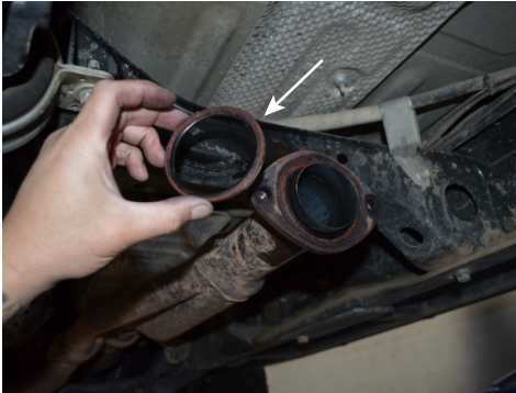
4. Remove the OEM donut gasket.
