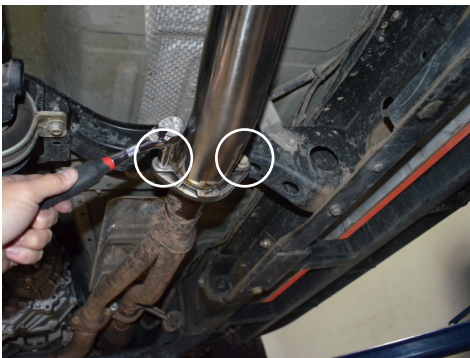
7. Secure the front pipe with the OEM bolts.
