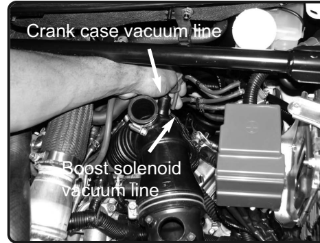
3. Disconnect the boost solenoid vacuum line and crank case vacuum line from the stock air duct. Also, loosen the clamp on the turbo side to disconnect the air duct.
