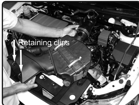
6. Remove the two front plastic retaining clips and continue to remove the entire OE air box assembly out with the air duct.
