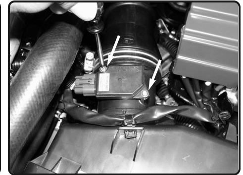
4. Loosen the screws, disconnect the MAF sensor harness and then remove the MAF sensor from the OE air box assembly.
